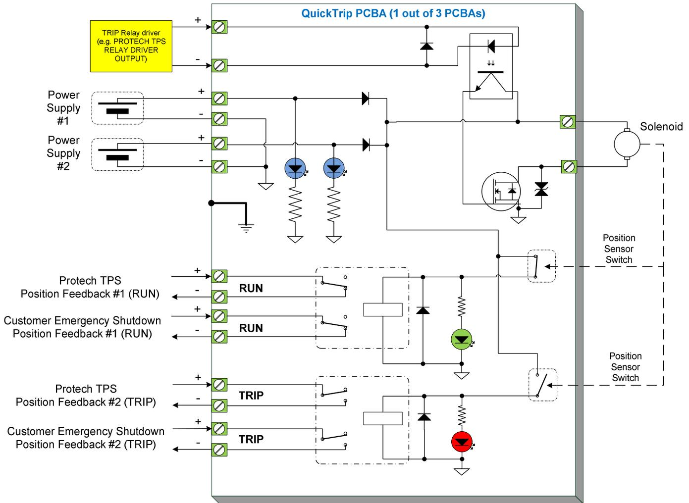
Figure 4. QuickTrip Module Electrical Schematic
