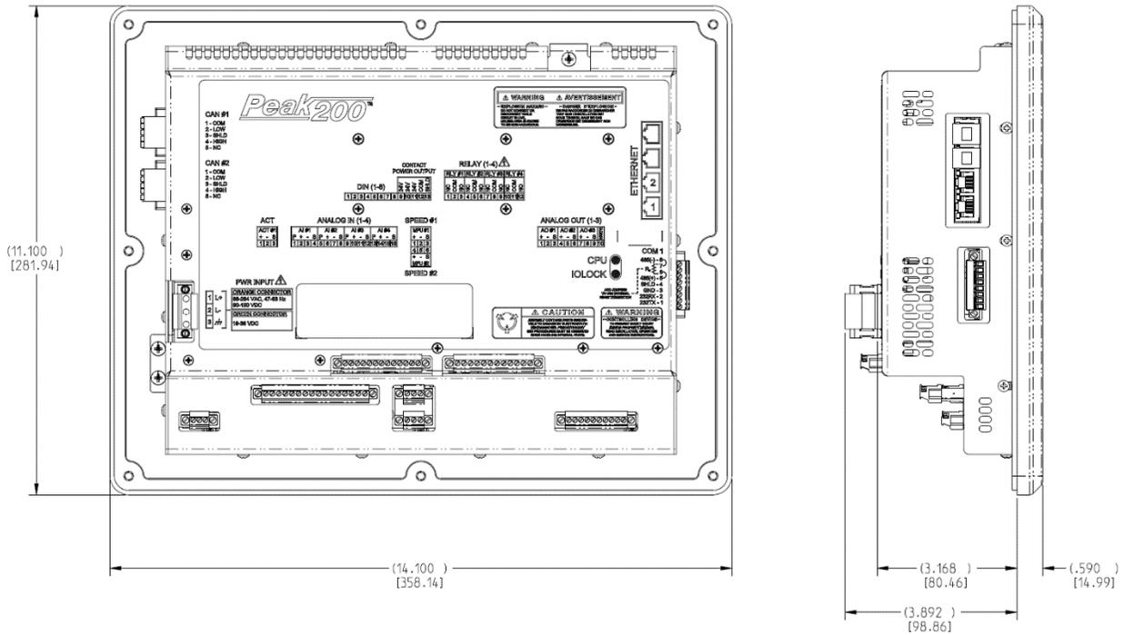
Figure 5. Peak200 Dimensions (Front Panel Mount Models)
