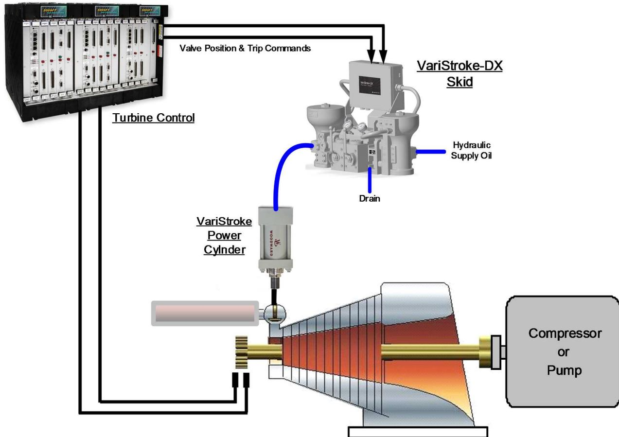
Figure 1. Typical VariStroke-DX Skid Applications
