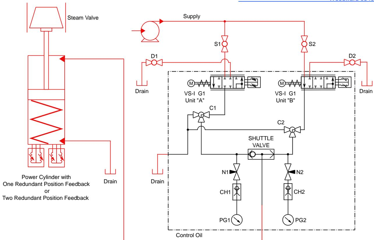
Figure 5. VariStroke-DX Skid Functional Diagram
