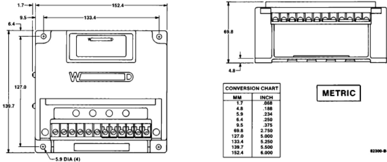
Figure 1-2. Outline Drawing for EPG 512/1712 and 524/1724 Speed Controls
