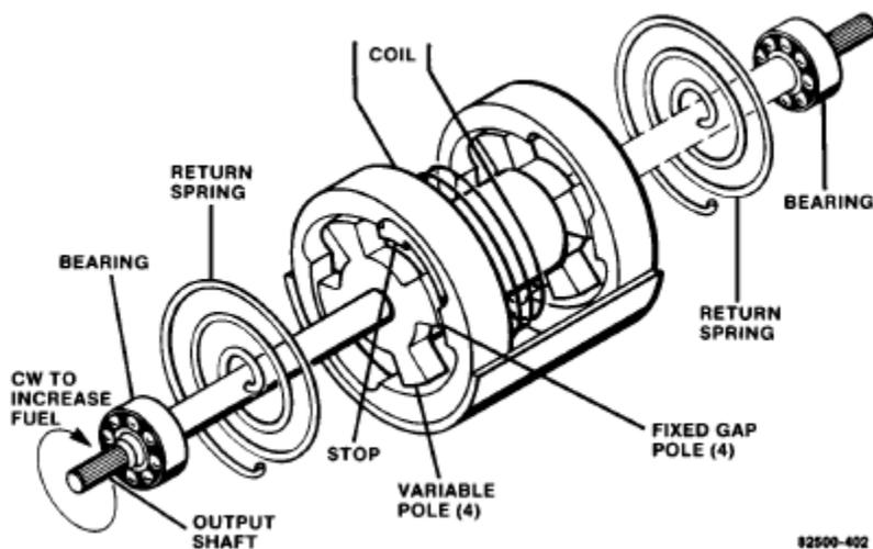
Figure 4-2. Actuator Schematic
