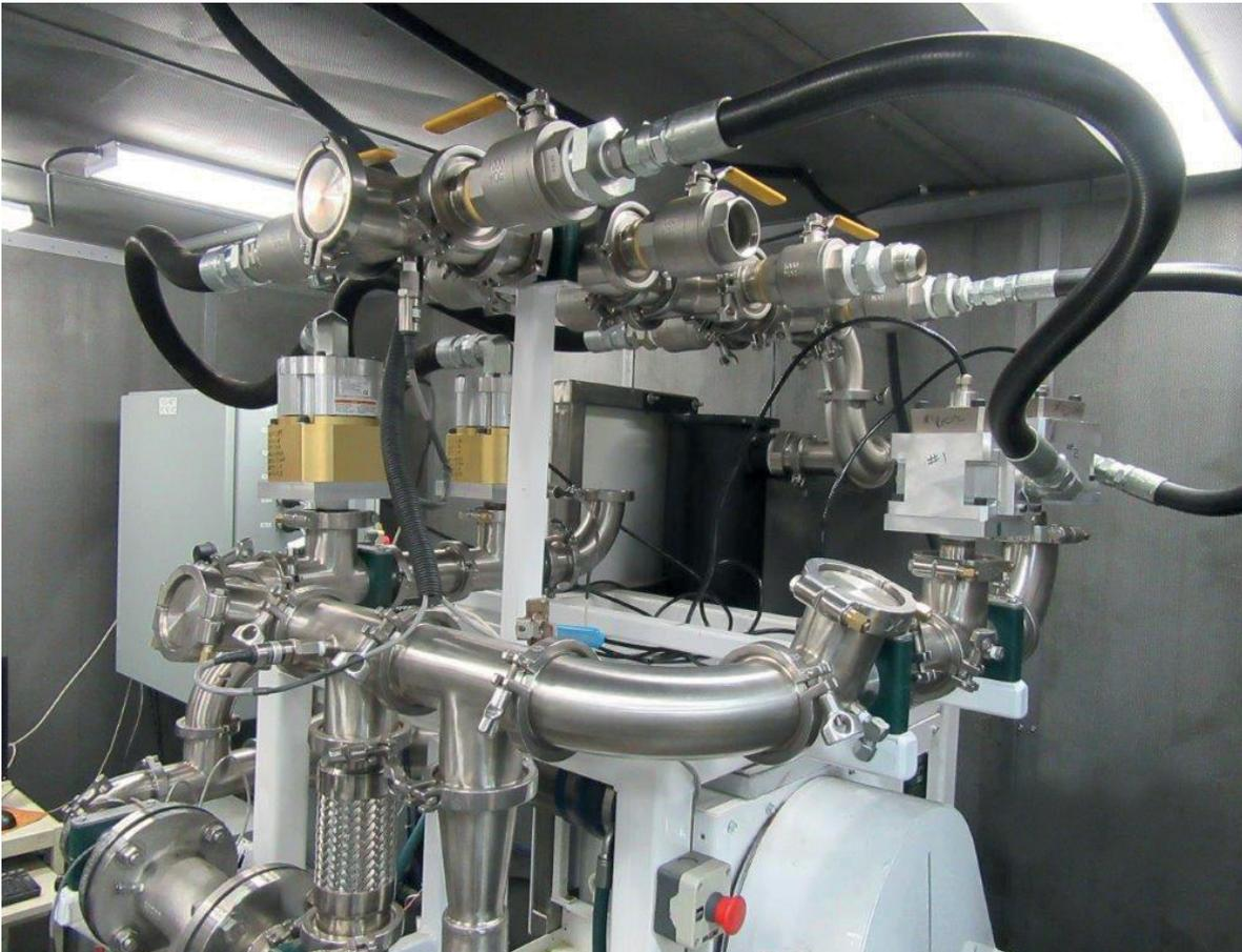
■ New fuels have called for a lengthy research and development process: Woodward's SOGAV250 and SOGAV65 on the testbench
